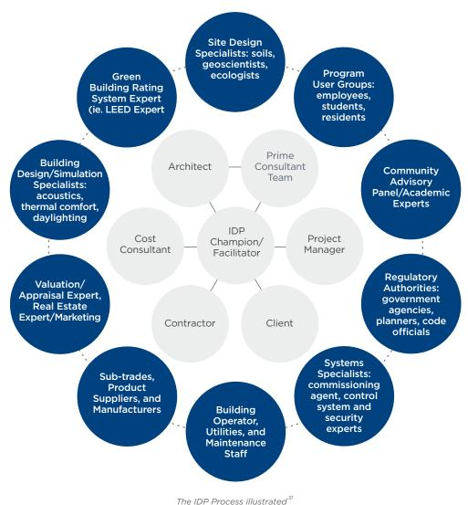
We have seen throughout the previous Drivers how facilities are systems of systems. That is, systems that functionally and operationally depend on each other and cannot be separated. While conventional project delivery treats each system discipline discretely, integrated design accepts this interdependency premise and strives to optimize performance over the whole facility life cycle.
